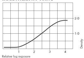
FP4 Plus roll film developed in ILFORD ILFOTEC HC (1+31) for 8 minutes at  $20^{\circ}\text{C}/68^{\circ}\text{F}$  with intermittent agitation. This curve is also representative of the 35mm and sheet film formats.
