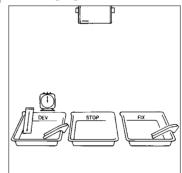
Set up your safelight (e.g. the ILFORD SL1 safelight) at least 1.2m/4ft from the developing dish. Lay out three processing dishes, label them DEV, STOP and FIX, two pairs of print tongs, and a clock for timing development. Then mix up the processing chemicals using water at about  $23^{\circ}C/73^{\circ}F$ . The aim is to process at a working temperature of  $20^{\circ}C/68^{\circ}F + /-1^{\circ}C/2^{\circ}F$ , so a few degrees are allowed for heat lost in mixing and cooling.
