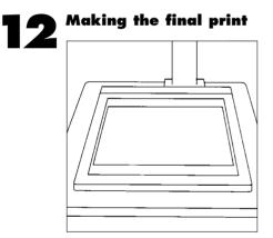
Switch the room light off and, by safelighting, position the easel under the enlarger to frame the print as you want it. Take out a new sheet of MULTIGRADE paper, and place this on the easel. Using the timer, give the paper the correct exposure worked out by examining the test print.
