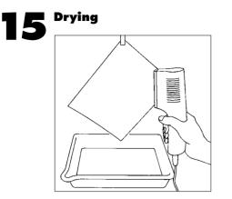
After the wash, drain the print and use a squeegee or sponge to remove any excess water. Attach a wooden or plastic clip to one corner, and hang the print over a drip tray to dry. Drying can be speeded up by using a hairdryer on a low setting, kept moving and about 30cm/1ft away from the print. MULTIGRADE prints dry naturally in a warm room in under 30 minutes.
