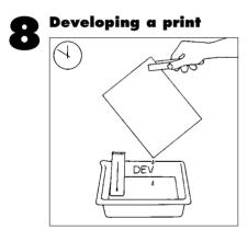
Check the thermometer in the dish of developer (20°C/68°F) and set the timer to zero. Slide the paper quickly and smoothly into the developer, making sure there are no air bubbles on the shiny surface. Start the timer. Rock the developer dish continuously backward and forward to send the solution gently over the print. After 50 seconds, use tongs to lift the paper out, and drain off the developer.
