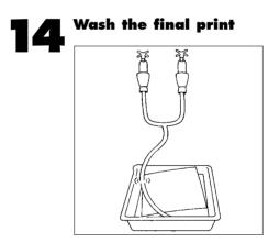
Wash the print for 2 minutes in a good flow of water ideally at about 20°C/68°F but cold water above 5°C/41°F will give adequate washing. Empty the wash tray a few times to ensure a complete change of wash water, or use rubber tubing to syphon water from the bottom of the tray.
