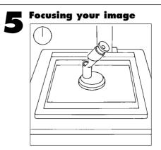
With the lens at full aperture, turn on the enlarger. Place an easel loaded with a spare piece of paper on the baseboard. Move the enlarger head to frame and focus the image. You can use a special 'focus finder' placed in the centre of the image to focus on the negative grain for the sharpest possible image.
