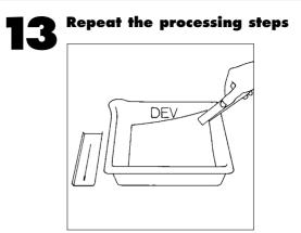
Repeat the processing steps (8-10) exactly as you did before. Again, check the temperature of the developer and time the development stage. If the developer has cooled more than a few degrees, warm it up by pouring it into a 600ml cylinder and running hot water over the outside of it. (The temperature of the stop and fix are not as critical.)
