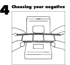
Choose the negative for printing, and make sure it is clean. Remove any dust with a puffer brush. Hold the negatives so you can read the edge numbers, then turn the negatives round (not over) so the numbers are furthest away from you. Place the negatives in the negative carrier of the enlarger. Slide the negative carrier into place. Switch on the safelight and switch off the roomlights.
