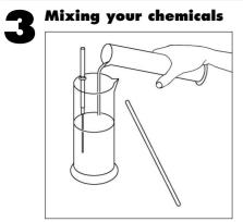
Mix up the developer solution 1+9 by measuring out 60ml of ILFORD MULTIGRADE developer in a 150ml cylinder, and adding this to 540ml of water in a 600ml cylinder. For the stop bath, add 30ml of ILFORD ILFOSTOP stop bath to 570ml of water (1+19). For fixing, add 150ml of ILFORD PAPER FIXER to 450ml of water (1+4). (This gives enough processing solutions to process about 40 20.3x25.4cm/8x10in MULTIGRADE RC prints).
