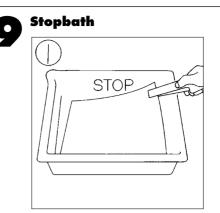
As one minute shows on the timer, quickly and smoothly slide the developed paper into the stop bath. take care not to contaminate the developer tongs with the stop bath. Rock the dish for about 30 seconds. Use the second pair of tongs (from the fixer) to lift the print while solution drains from it, and transfer it to the dish of ILFORD RAPID FIXER solution. (The timing of this step is not critical.)
