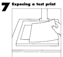
With the safelight on, and the room lights off, put a sheet of MULTIGRADE paper into the easel, shiny side up. (Reseal the packet carefully.) You are now ready to make a test print. Switch on the enlarger lamp and expose the whole sheet for two seconds. Cover one-quarter of the sheet with opaque card, and expose the rest for another 2 seconds. Cover half of it, and expose the rest for another 4 seconds. Cover three-quarters, and expose the last part for another 8 seconds.
